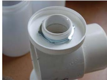
22. Drill 1⅞" hole in a jar lid. Place this on the 1½" adapter and secure with locknut.
