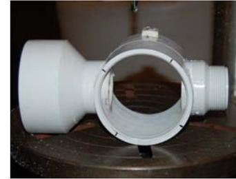
19. Glue the adapter and coupling into the 3" coupling.
