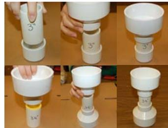
28. **Po' Gizmo:** cement 3" pipe to cap. Turn over and cement coupling.
