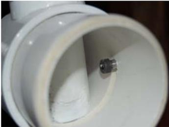
21. Put 3" pipe into 3" coupling so the slot lines up with the thread insert. Screw the shoulder screw in from the inside.
