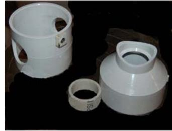
18. Cut a 1½" pipe the length to fit into the coupling (step 16) and extend into the 3" coupling. Glue this pipe into coupling.
