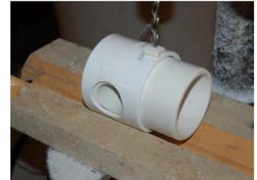
6. Cut off excess 1 1/2" pipe and sand flush with 3" pipe. Save cutoff piece for future use.
