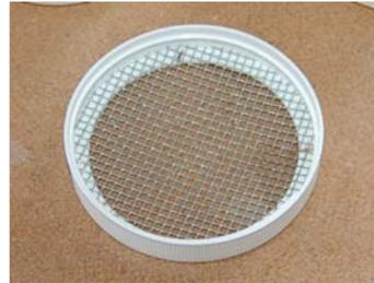
23. Drill a 3" hole in a jar lid. Cut a piece of 8x8 hardware cloth to fit in the lid. It is helpful to have multiple jars and lids to do multiple samples.
