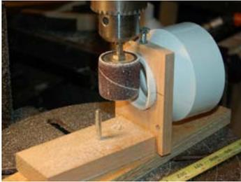
16. Sand the 1½" end of the 1½" x 3" coupling to match the outside curve of the 3" coupling.
