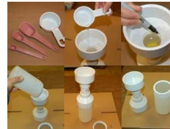
29. Measure 100 mL water as explained in poster 168. Pour in and mark line at the water level.
